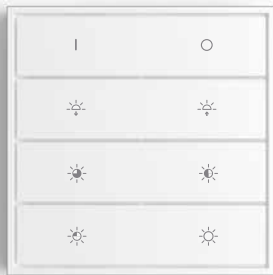
OPT-1DIM Rolling Code 433,92MHz radiotransmitter, 1 channel, functions: On-Off, dimmer up/down, light level selection 25%-50%-75%-100%. Battery CR2450
